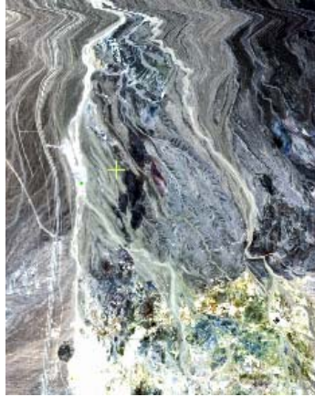
Figure 4.2.1: Distortion caused by aircraft roll is apparent in the upper portion of this image
