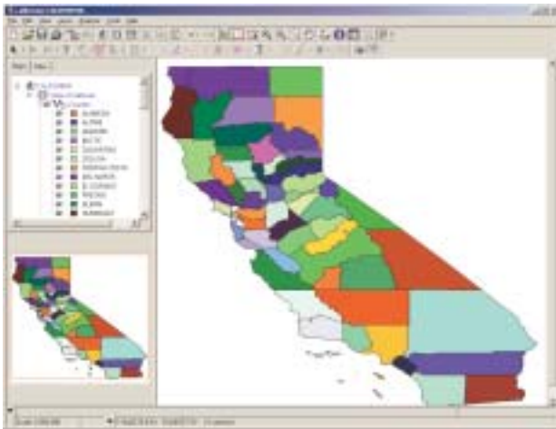
Vector layer legend in MAPS Tab tree list showing counties within the state of California, USA
